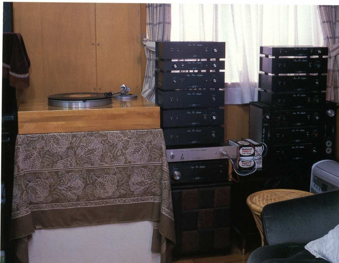
Turntable unit is out, on a concrete block up directly from the floor foundation. Turntable is equipped with a DC amplifier control. On right, Successive pre-amp are piled up
